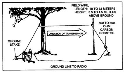
Figure 7-10. Long-wire antenna.
