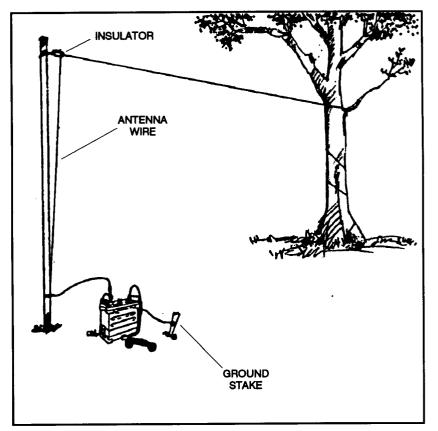
Figure 7-5. End-fed half-wave antenna.
