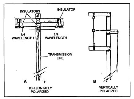
Figure 7-7. Center-fed half-wave antenna, supported.
