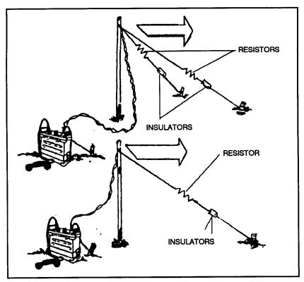
Figure 7-12. Sloping-V antenna.
