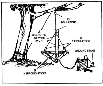
Figure 7-13. Expedient 292-type antenna.
