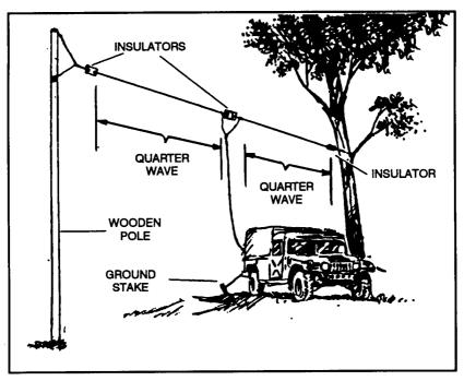
Figure 7-6. Center-fed half-wave doublet antenna.
